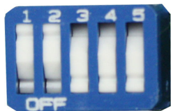
Figure 2-3: DIP switch set to Decimal Address 3
