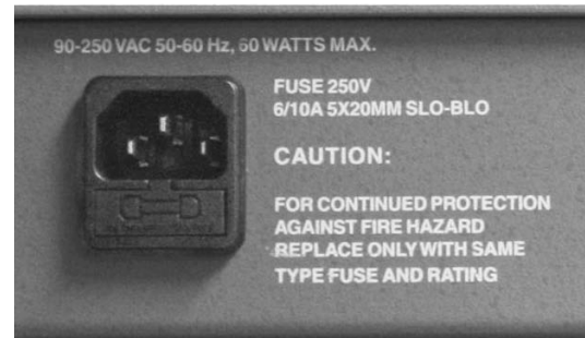
Figure 2-1: Input power module with a drawer for the input fuse
