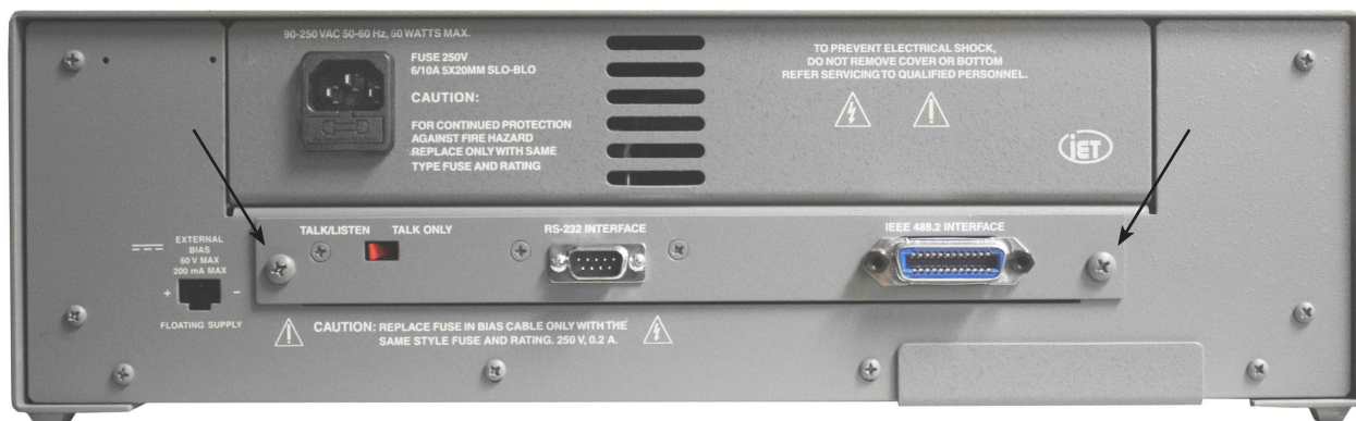
Figure 5-1: Screws holding the interface assembly on the rear panel
